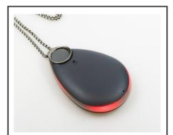
The light-ring around Chiptech GO will flash red to let you know an alert is being sent to the Alarm Receiving Centre (ARC) A voice message will play, "Help alert in progress."
