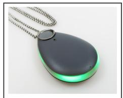
When an operator ends the call Chiptech GO will flash green to indicate that the ARC can still call back, and your location continues to be sent. Chiptech GO automatically stops reporting your location after a period of time, the green lights
